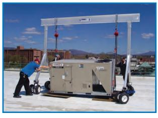
With systems as light as 116 pounds, just one workers can typically carry, assemble, and precisely position a Spanco Aluminum Gantry Crane almost anywhere — including rooftops. Designed to easily fit into or on top of most service trucks, these lightweight gantries carry up to 3 tons and are popular with contractors and in the HVAC industry.
