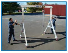
Two workers adjusting the height on an aluminum gantry crane using a Lug-All® Winch Hoist.
