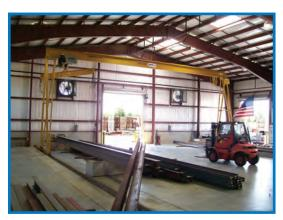
A Spanco Motorized 7.5-ton PF-Series Gantry Crane used to move truckloads of long steel beams at a building material supply center
