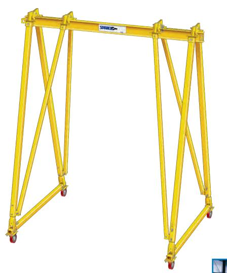
**Superior Stability:** Superior engineering leaves the I-beam free to pivot as it self-centers over the load, while the "A"-frame design keeps the rest of the crane perfectly stable. Main legs, brace legs, and caster frames are made of heavy-gauge, square tubing with zinc-plated hardware.
