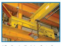
A Top-Running Single Leg Gantry Crane traveling along a ceiling-mounted runway.
