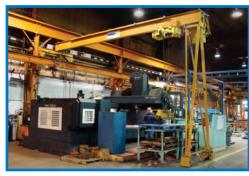
A Spanco 3-Ton Single Leg Gantry Crane with one end supported overhead and one end traveling along the floor.
