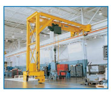
A Spanco Motorized 5-ton Wide-Flange Single-Leg Gantry Crane with an overall span of 20 feet and 15 feet under the beam.
