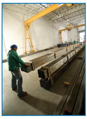
Workers using two Motorized Spanco PF-Series Gantry Cranes to load and transfer steel bundles.
