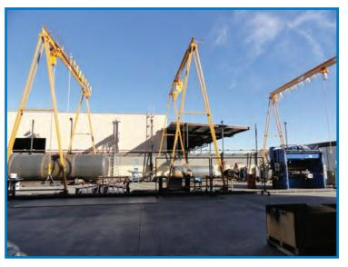
Three track-mounted PF-Series Gantry Cranes mounted over rail cars for easy maintenance and repair. The track mount ensures smooth travel over a fixed route for increased productivity and ease-of-use.
