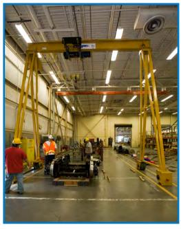
A Spanco 7.5-ton PF-Series Gantry Crane with a Guide Angle Power Drive Kit & Guide Rollers for high-volume, high-capacity travel along a fixed path.
