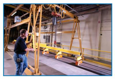
Custom Spanco Motorized PF-Series Gantry Crane System
